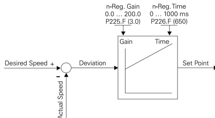
The PI-controller's job is to make speed corrections quickly a minimal amount of overshoot and oscillation. Parameter P225 (gain) and parameter P226 (time) are used to tune the PI-controller's performance. The end result should be a fast response time with about a 43% initial overshoot. The motor should then settle in to the new desired speed.
