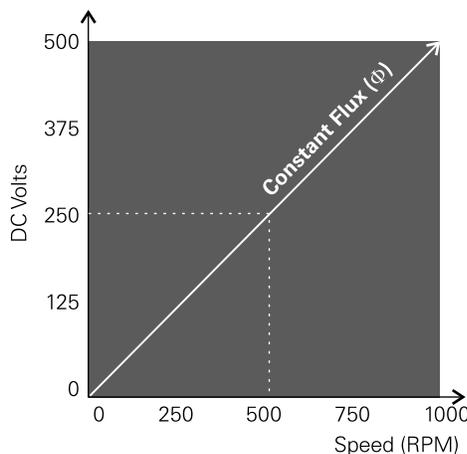
$$\text{Speed } (n) = \frac{V_a - (I_a R_a)}{K_t \Phi}$$
