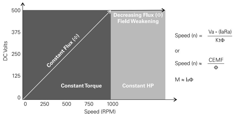
Horsepower is said to be constant because speed (N) increases and torque (M) decreases in proportion.
