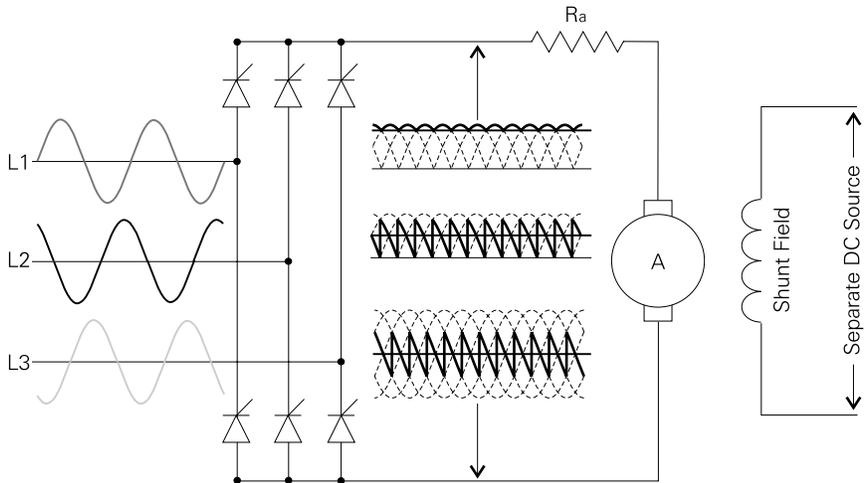
It is important to note that the voltage applied to a DC motor be no greater than the rated nameplate. Armature windings are commonly wound for 500 VDC. The control logic in the drive must be adjusted to limit available DC voltage to 0 - 500 VDC. Likewise, the shunt field must be limited to the motor's nameplate value.
