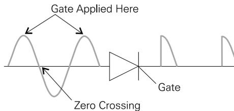
The amount of rectified DC voltage can be controlled by timing the input to the gate. Applying current on the gate at the beginning of the sinewave results in a higher average voltage applied to the motor. Applying current on the gate later in the sinewave results in a lower average voltage applied to the motor.
