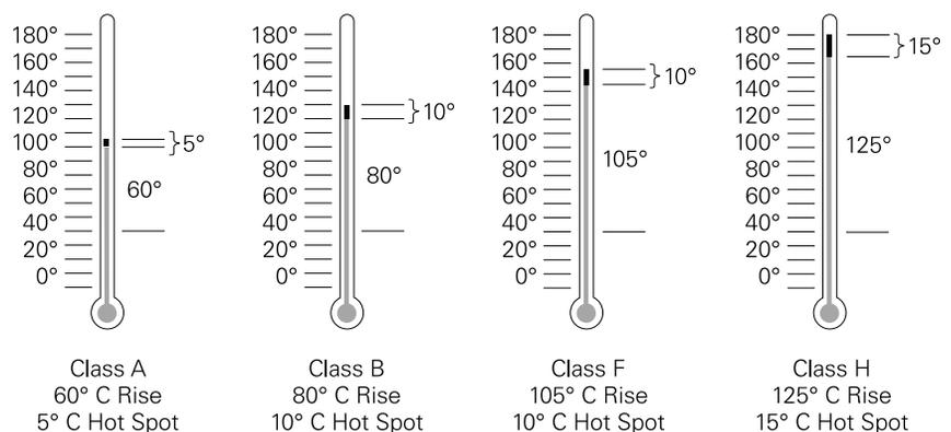
The operating temperature of a motor is important to efficient operation and long life. Operating a motor above the limits of the insulation class reduces the motor's life expectancy. A 10°C increase in the operating temperature can decrease the life expectancy of a motor by as much as 50%. In addition, excess heat increases brush wear.
