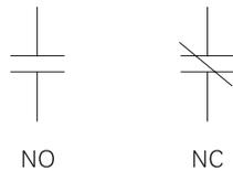
The standard method of showing a contact is to indicate the circuit condition produced when the actuating device is in the de-energized state. For example, in the following illustration a relay is used as the actuating device. The contacts are shown as normally open, meaning the contacts are open when the relay is de-energized. A complete path of current does not exist and the light is off.
