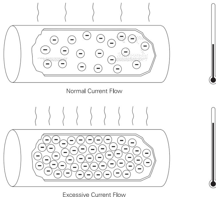
Excessive current is referred to as **overcurrent**. An overcurrent may result from a short circuit, overload, or ground fault.
