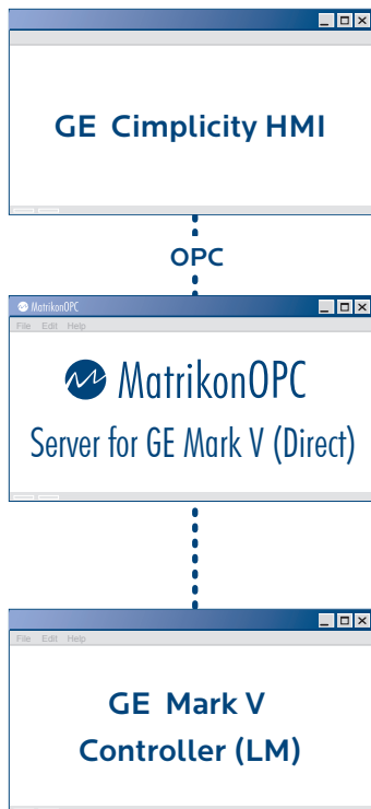
Figure 2 - Direct OPC Server Connection to GE-Mark V
